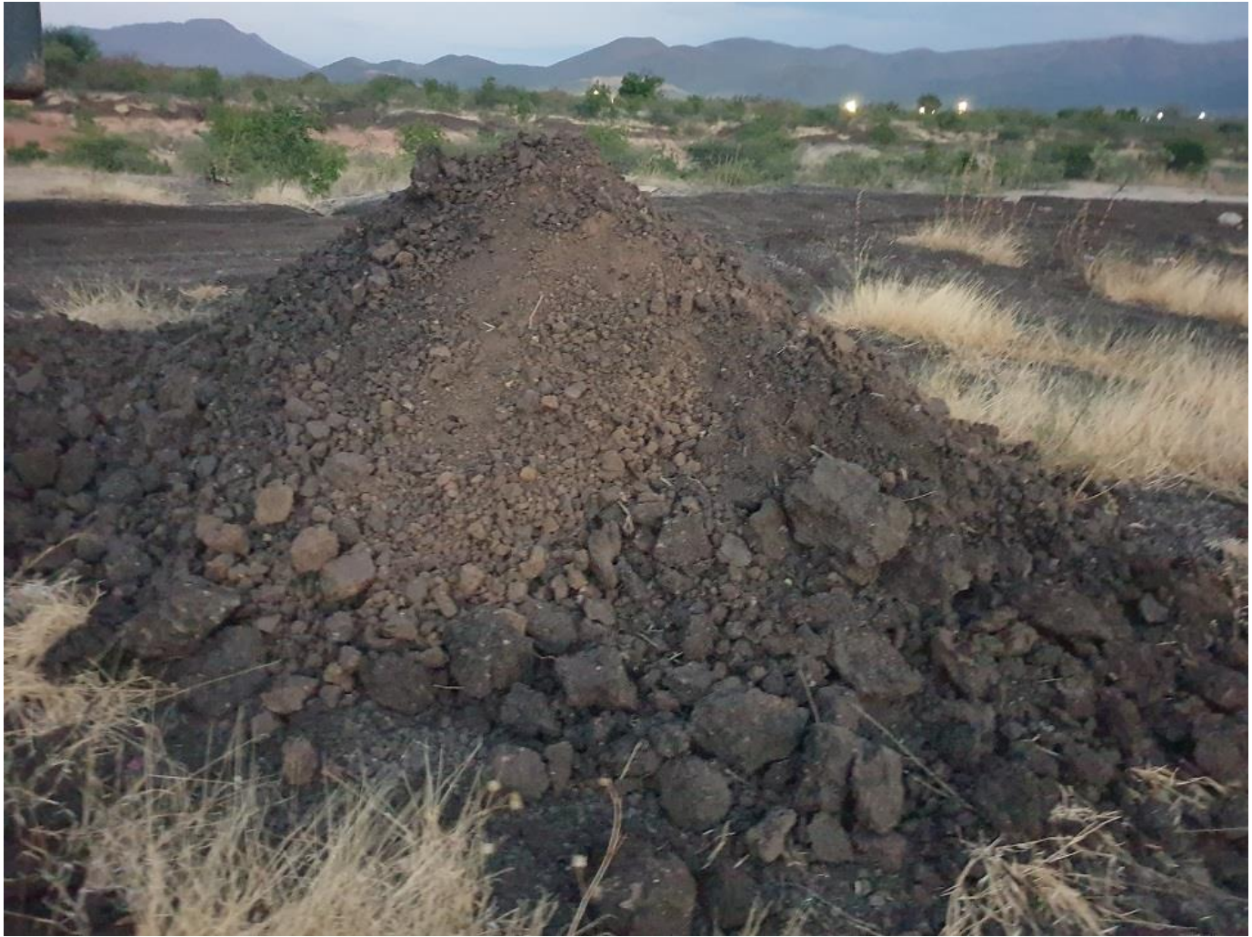
Plate 21. Spoil from test pit HRC/4.
